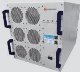
4KW S-Band (2.0-4.0GHz) Solid State Pulse Amplifier-
