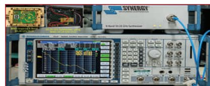
▲ Fig. 4 Phase noise measurement of a 10.24 GHz MMS DRO.
